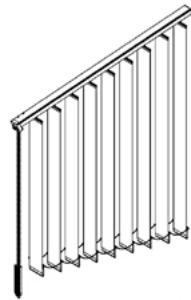
diagonal rail on adjustable hangers (the length of each slat can be adjusted)
